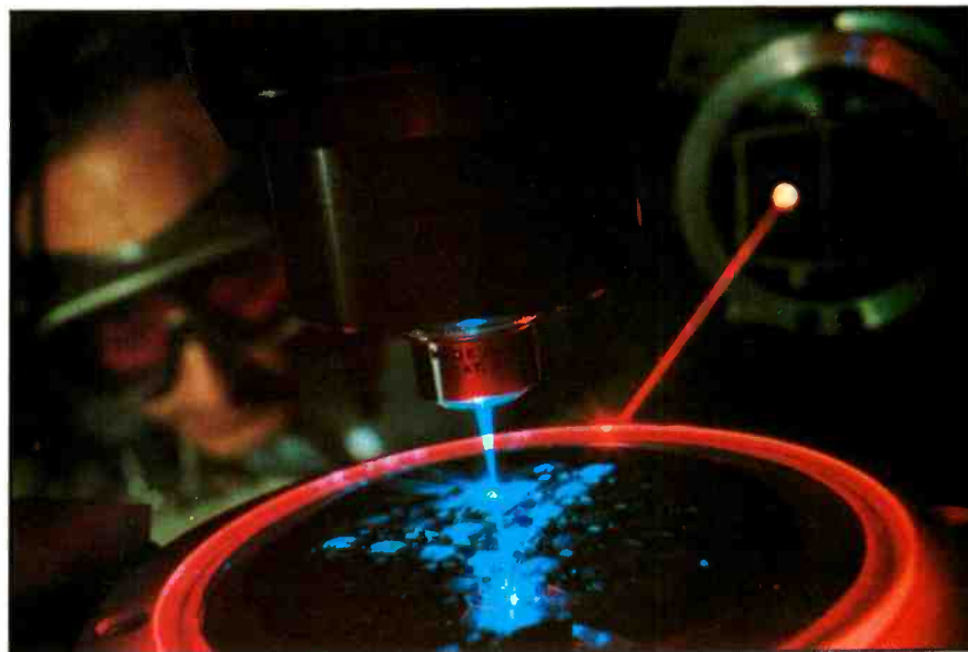
An intense beam of light from a laser scribes microscopic lines that connect integrated circuits on the surface of a material.
