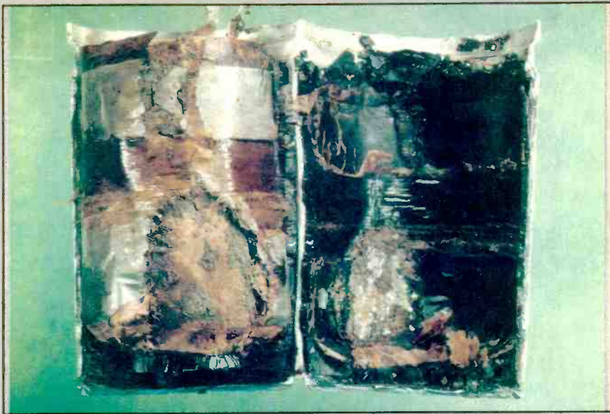
Figure 11. Here, there is anodic corrosion of an aluminum capacitor.
